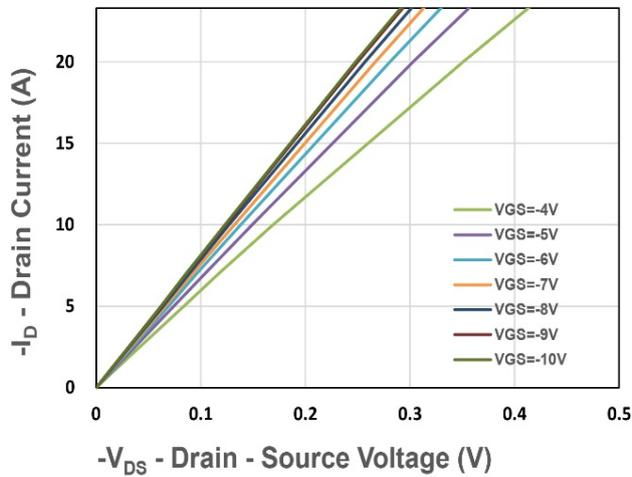
**Figure 1. Output Characteristics**
